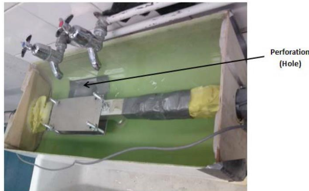
Figure 2.3: Damaged segment of ship model
